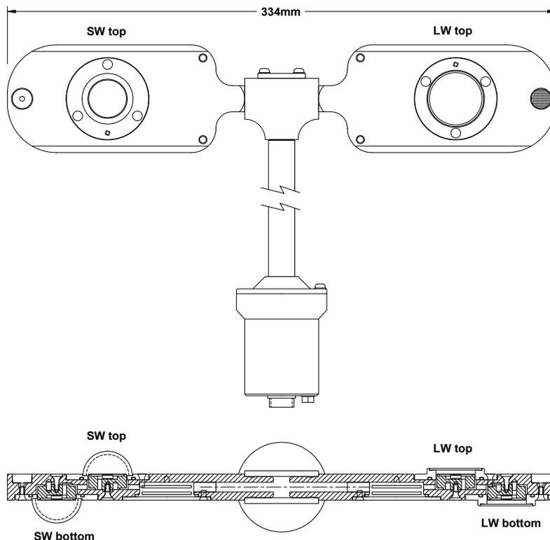
**Maintenance.** Keep the domes and windows clean and free from debris; use water and mild detergent only. Calibration is recommended every two years. Desiccant is inside the cylinder at the end of the handle; it should be replenished at calibration.
