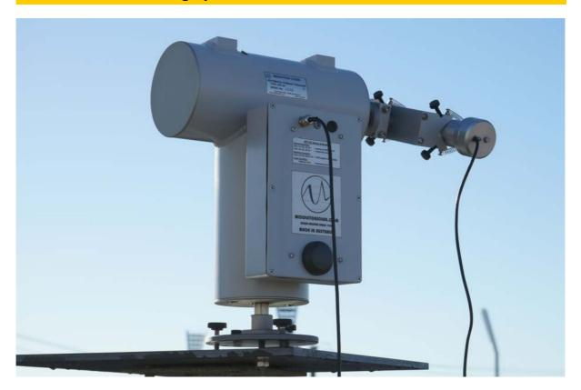
The Middleton Solar APT-02 is a 2-axis tracker to automatically point solar radiometers at the sun throughout the day. The APT-02 is a simple Passive Tracker without the closed-loop control of the fully active AST-02/3 Tracker from which it is derived.
