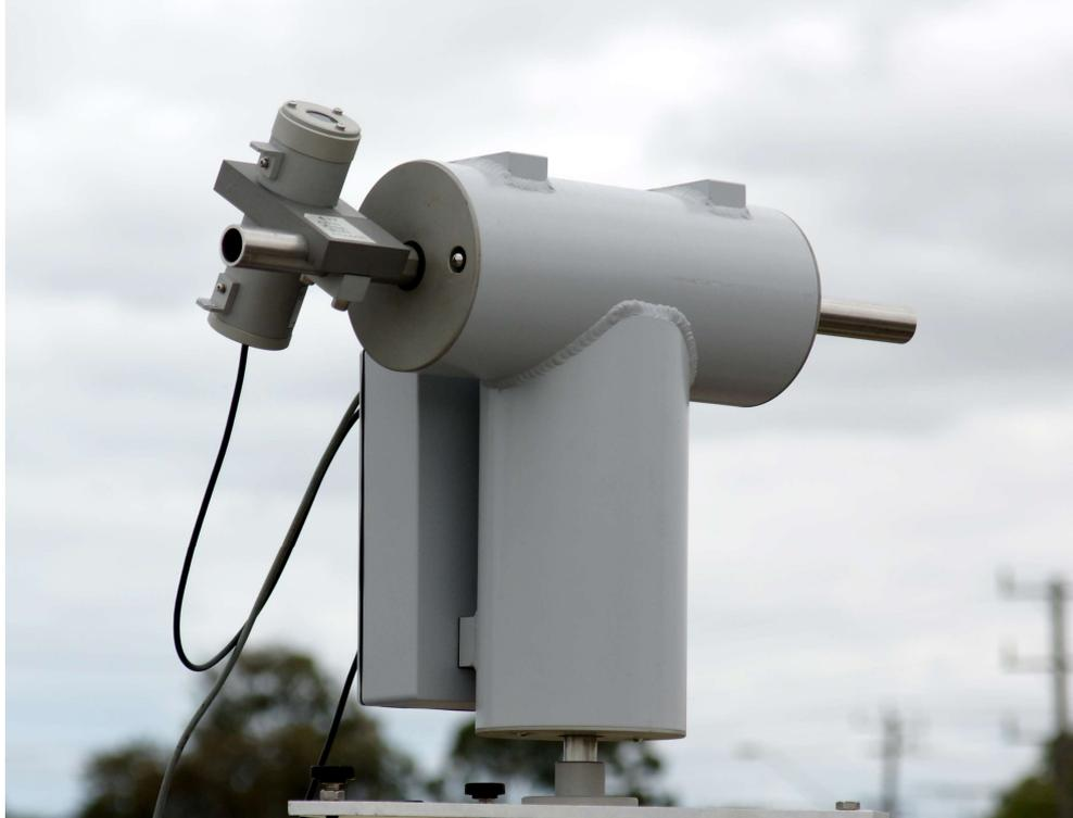
The Middleton Solar AST-02/3/3T is an active sun tracking system for solar instruments used to measure direct and diffuse irradiance. The AST-02 has a single elevation shaft. The AST-03 has two coaxial elevation shafts mechanically locked together, and the AST-03T version has two coaxial elevation shafts that are controlled separately to facilitate shade/un-shade and alignment testing.
