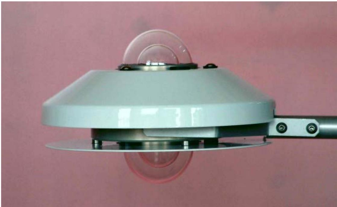
The Middleton EQ16 Pyrano-Albedometer is a dual head version of the Middleton EQ08 First Class Pyranometer. It is for the measurement of the ratio of upward to downward solar radiation flux density on a plane surface. The EQ16 has a direct microvolt output, and the EQ16-E version has in-built signal amplifiers.
