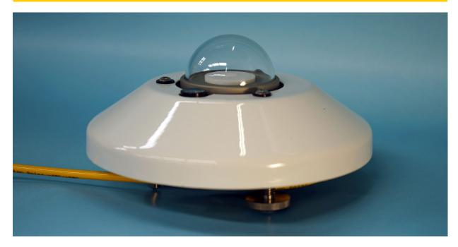
The Middleton Solar ER08-S is for measuring solar Global Horizontal Irradiance (GHI). It exceeds the ISO specifications for a Fast Response Spectrally Flat Pyranometer of Class B or Class A, and uses a proprietary Integrating Cavity Thermopile to achieve very low zero off-sets, even when internally heated. The ER08-S has a passive microvolt output. The ER08-SE version has an in-built signal amplifier to give a millivolt output for easy signal measurement.
