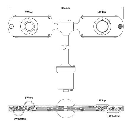
**Maintenance.** Keep the domes and windows clean and free from debris; use water and mild detergent only. Calibration is recommended every two years. Desiccant is inside the cylinder at the end of the handle; it should be replenished at calibration.
