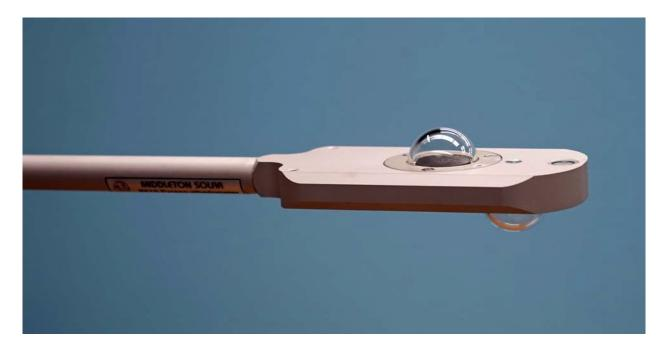
The Middleton Solar SK16 Pyrano-albedometer is for measuring albedo, the ratio of upward to downward solar radiation through a horizontal plane. The SK16 has separate upper and lower thermoelectric sensors each shielded by a glass dome window. The domes are transparent to shortwave solar radiation from the sun (top sensor), and shortwave reflected from the Earth surface (bottom sensor). The sensors are matched for response time, and their collector surfaces are parallel.
