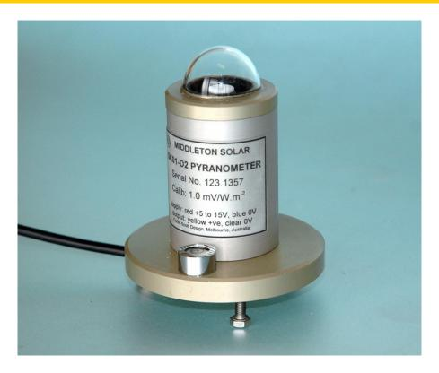
The SK01-D2 is a simple pyranometer for measuring total solar global radiation on a horizontal surface. The SK01-DP2 version incorporates a special filter to limit its sensitivity to the Photosynthetically Active Radiation region of the solar spectrum (400-700nm).
